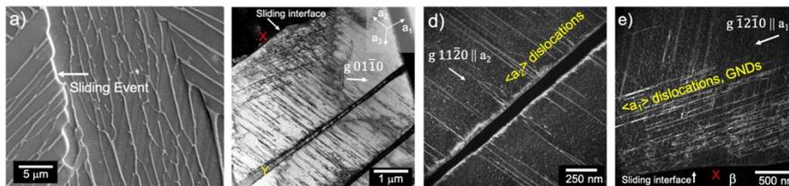
**Figure 1:** Sliding event in (a), the two responsible glide systems in the BF image of (b) and corresponding WBDF images of the  $\langle a_2 \rangle$  system and  $\langle a_1 \rangle$  system in (d) and (e), respectively.
