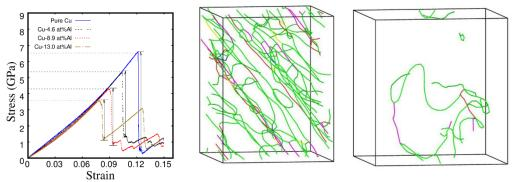
Stress strain curves and dislocation microstructure for Cu and Cu-13 at% Al
