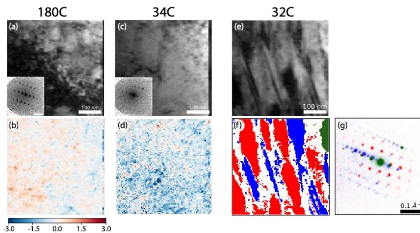
Fig.1 (a,b,e) bright field images of NiTi at the indicated temperature, (b,d) percent strain along the  $\langle 01\bar{1} \rangle_{B2}$  direction (f) map of martensite (blue and red) and austenite (green) phases at 32C, and (c) overlaid diffraction patterns of each phase in (b)
