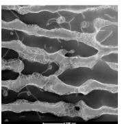
Fig. 1: DF-STEM image of rafted ERBO1 superalloy microstructure after uniaxial creep exposure at 1223 K, 300 MPa and 4% accumulated strain.  $\gamma$  and  $\gamma'$  phases shown in bright and dark contrast, respectively.
