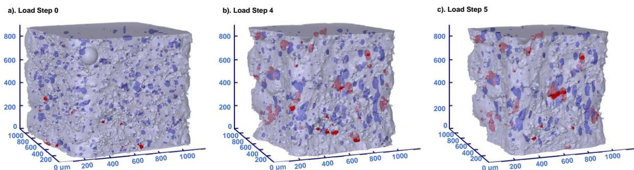
Figure 1: Three-dimensional reconstructed pore distribution for sample 2 at a). Load Step 0 (as-built condition), b). Load Step 4, and c). Load Step 5 (final failure).
